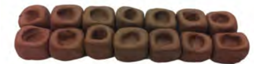
Compressed Mud Block Hollow section 30x30x30cm
